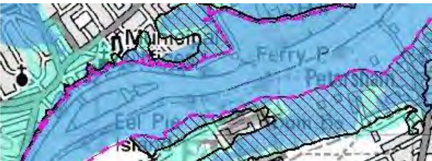
Flood Risk at Ham. The darker blue indicates the 1 in a 100 flood event with the dashed lines showing the land protected from a tidal flood by the Thames Barrier. Inside the dashed purple line there is no statutory flood protection although at present the Thames Barrier can be used to protect against a fluvial flood event but it is anticipated that this operation will decline over the coming decades
