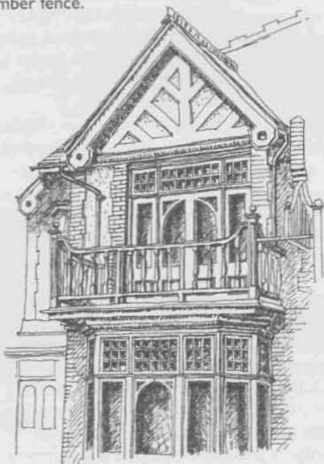
Balcony detail, nos. 16-22 (even) Seymour Road
